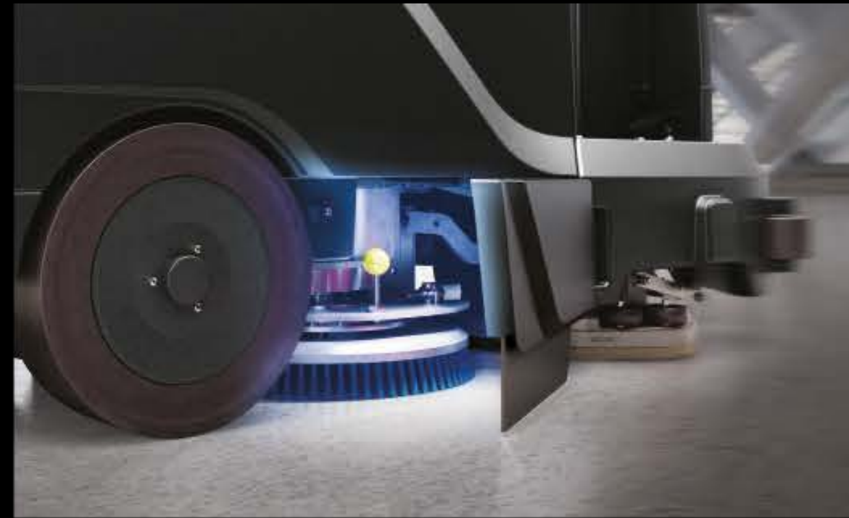
The exclusive lights pack offers increased visibility of the parts which could require operator inspection, illuminating the relative zones with LED lights
