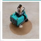
The compact Tigra sweeper has a reduced turning radius (950 mm), which enables cleaning in tight spaces which are difficult to access.
